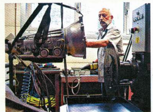
Dimo prepares to dyno-test a transmission.
